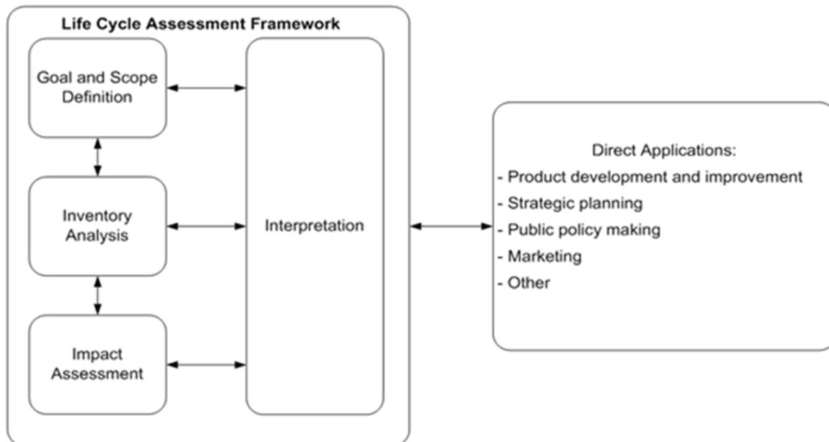
**Figure 1. Stages of an LCA (ISO, 2006).**
