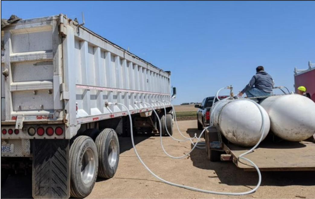
Figure 6: 1000-gallon tanks hooked up to CO2 ports on dump trailer to run gas in
