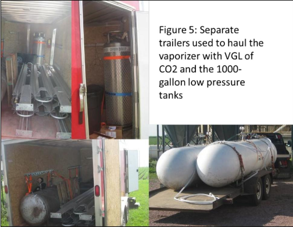
Figure 5: Separate trailers used to haul the vaporizer with VGL of CO2 and the 1000-gallon low pressure tanks
