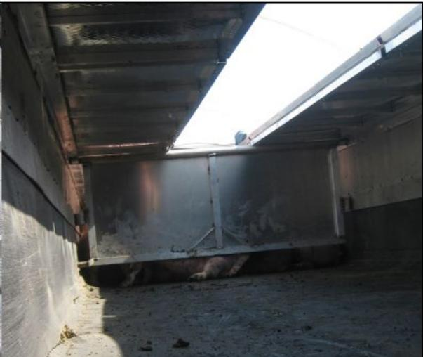
Figure 3: View of swing gate placed after trailer is filled halfway
