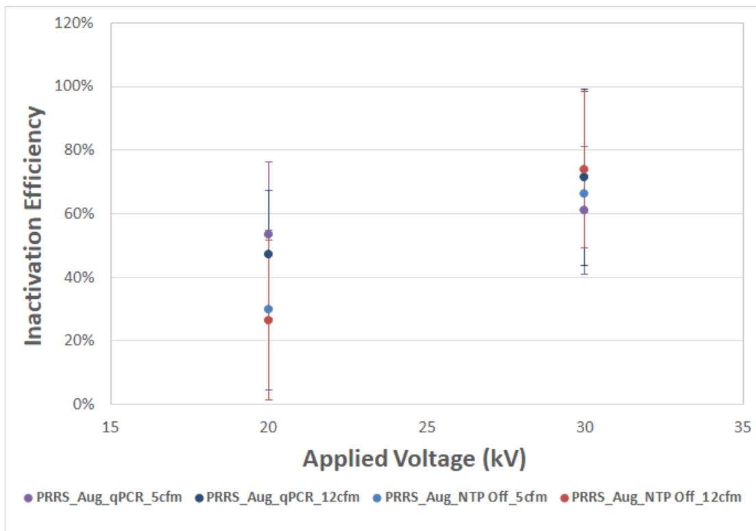
**Figure 4.** Results of phase 2 (August) PRRSv inactivation by NTP treatment at two air flow rates (5 and 12 cfm) and two voltages (20 and 30 kV, corresponding to 1.7 and 23 W, respectively). Compared are the results of two different methods for calculating inactivation efficiency: reduction in TCID<sub>50</sub> based on pre-
