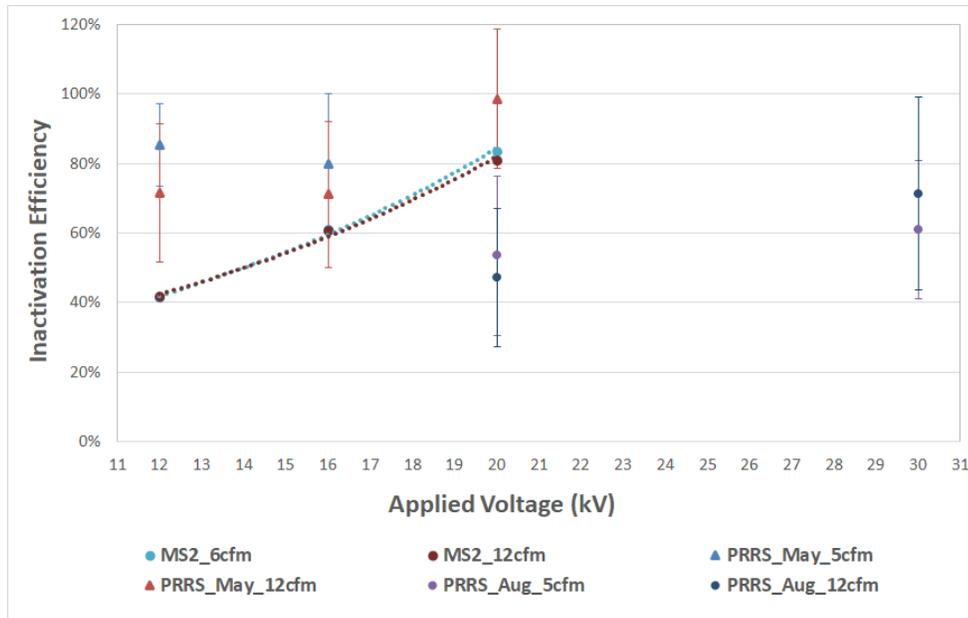
**Figure 3.** Comparison of phase 1 (May) and phase 2 (August) PRRSv inactivation by NTP treatment at two air flow rates (5 or 6 cfm and 12 cfm) and four voltages (12, 16, 20, and 30 kV), as compared to earlier results for MS2 phase inactivation at the same conditions (30 kV not shown).
