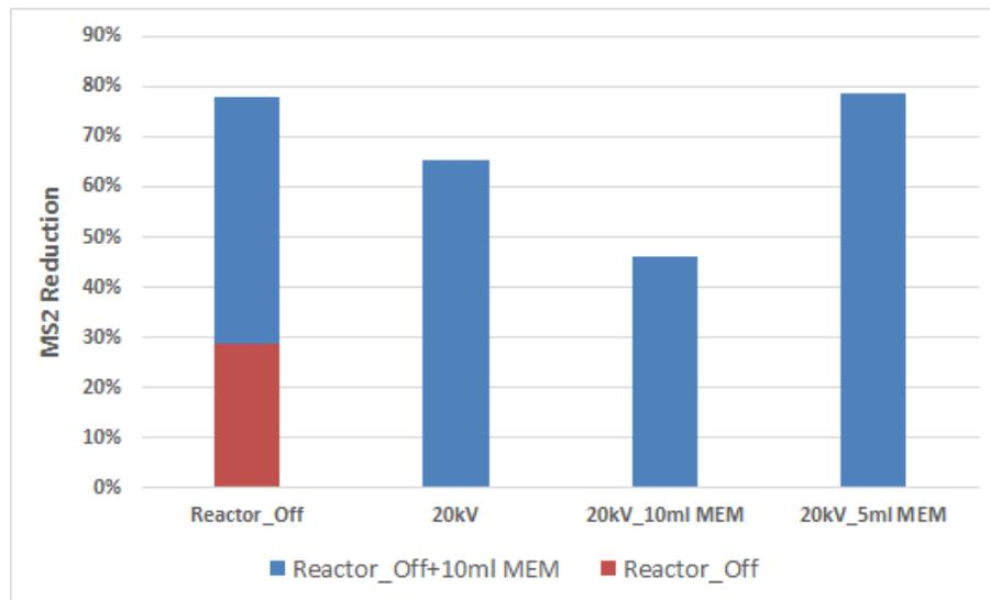
**Figure 6.** Results showing reduction (filtration + inactivation) of MS2 phage in response to 10 ml and 20 ml of MEM added to and held within the NTP packed bed. MEM was added to the packed bed first, before introduction of MS2 phage, aerosolized from VDB solution.
