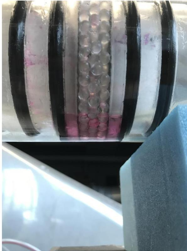
**Figure 5.** Photo showing the accumulation of MEM (pink liquid) after a 20 minute test, the result of incomplete evaporation of PRRSv-bearing MEM droplets before reaching the packed bed NTP reactor.
