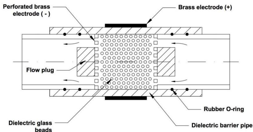
**Figure 2.** Schematic of the DBD packed-bed NTP reactor.
