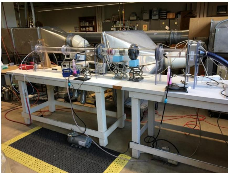
**Figure 1.** Photograph of the small-scale wind tunnel setup at Univ. of Minnesota with the NTP reactor mounted in the middle test section. The inlet is on the left side and the flow goes from left to right through the tunnel and HEPA filter where it is drawn out through a vacuum blower (not shown).
