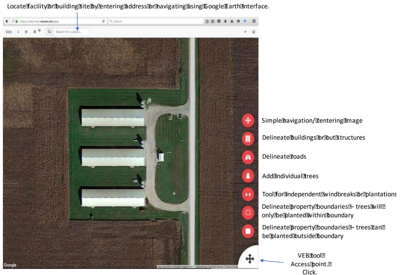
Figure 1. Description and example of the VEB-econ tool applications and online GIS interface.
