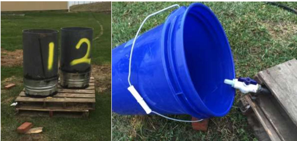
Figure 2. The complete soil columns set upright on the left. The metal tubs below the PVC are filled with sand and small gravel to encourage quick and complete drainage from the column. On the right is a close up of the ball valve that drains from the bottom of the column.
