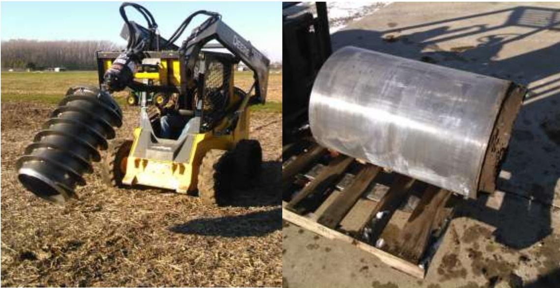
Figure 1. The soil-coring machine used to extract 20-inch soil columns is shown on the left. It is attached to a skid steer with a post-hole digger hydraulic motor. On the right, a soil column in the PVC sleeve
