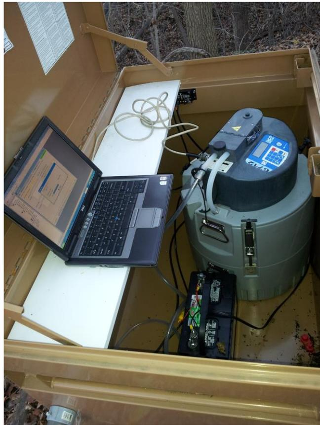
Figure 4: ISCO Portable Sampler placed in the job-box.
