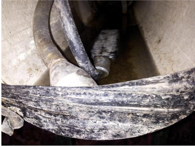
Figure 3: Area velocity flow sensor placed in the tile outlet along with ISCO sampler intake.
