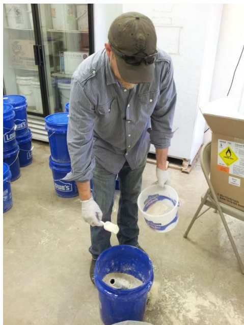
Figure 16. Farm scale - premixing of weighted ratio (~23.5:1 w/w) of soybean peroxidase treatment and \text{CaO}_2 catalysts.
