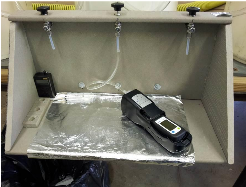
Figure 10. Drager portable gas analyzer used to measure \text{NH}_3 and \text{H}_2\text{S} from the vent line of the manure storage reactor via the gas sampling station.
