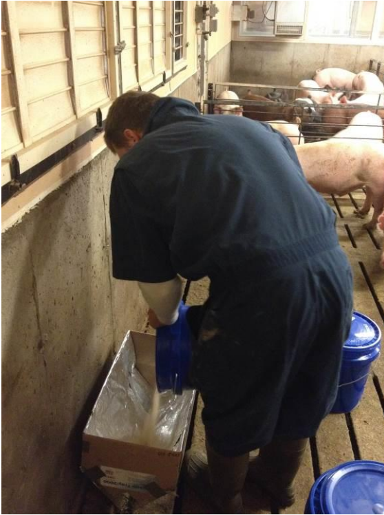
Figure 17. Farm scale - application of premixed soybean peroxidase treatment and \text{CaO}_2 catalysts through slats to the manure pit. Special funnel device was assembled to accelerate the application, to minimize losses and to apply treatment uniformly over the entire manure pit surface area.
