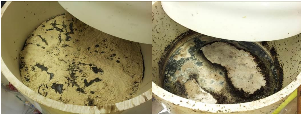
Figure 21: Simulated manure storage treated with 2.28 kg/m 2 SBP dose. Left: Day 14 after treatment, Right: Day 137 after treatment.
