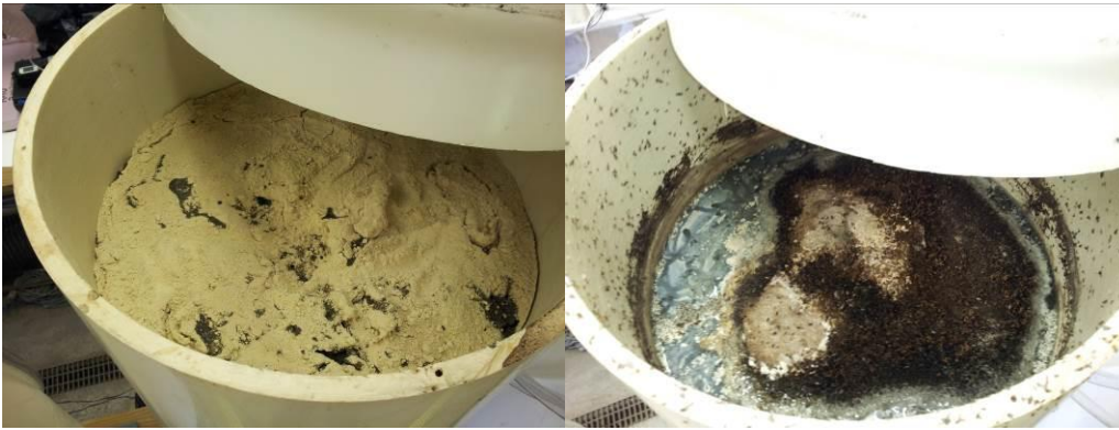
Figure 22: Simulated manure storage treated with 4.57 \text{ kg/m}^2 SBP dose. Left: Day 14 after treatment, Right: Day 137 after treatment.
