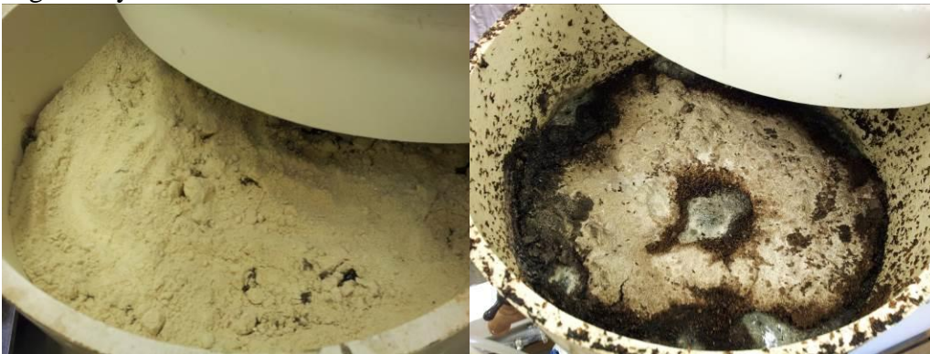
Figure 24: Simulated manure storage treated with 45.7 \text{ kg/m}^2 SBP dose. Left: Day 14 after treatment, Right: Day 137 after treatment. This relatively heavy layer of SBP had forced the SBP to crack the crust and roll into the top layer during periodic additions of “fresh” manure. This resulted in less manure surface coverage with the largest SBP dose over time.
