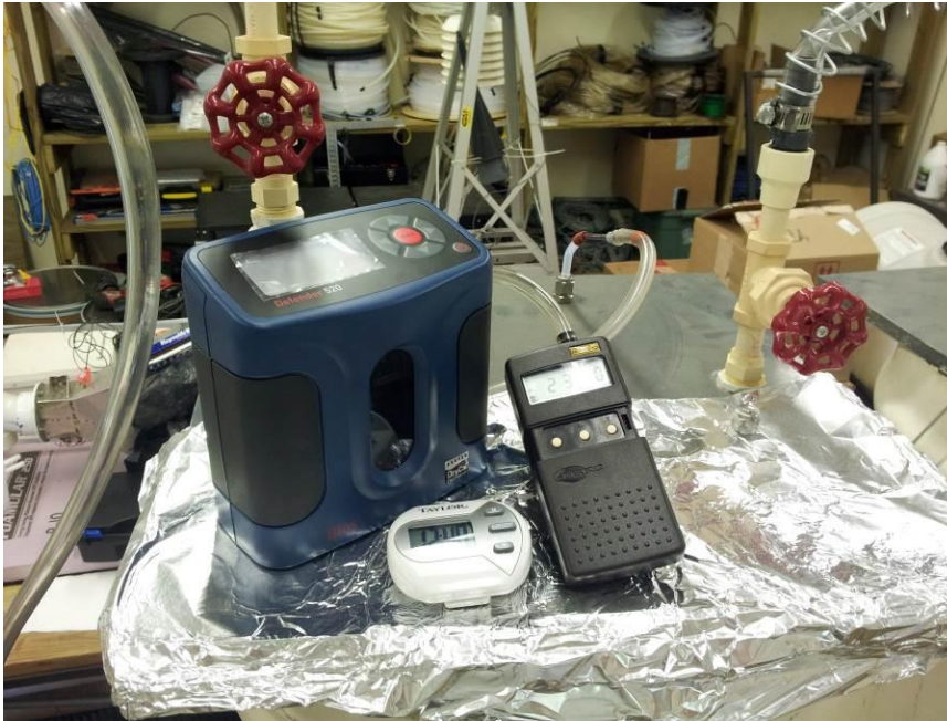
Figure 9. Pilot scale sampling setup for VOCs collection via sorbent tubes. Sampling pump pulls gas sample from the reactor vent line through the sorbent tube (4 mm O.D., 0.10 m long, packed with Tenax TA) and the gas flow rate is monitored via inline flow meter for the predetermined sampling time. Total gas sample volume can be estimated as a product of measured flow rate and sampling time.
