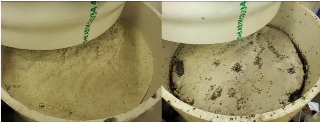
Figure 23: Simulated manure storage treated with 22.8 \text{ kg/m}^2 SBP dose. Left: Day 14 after treatment, Right: Day 137 after treatment.
