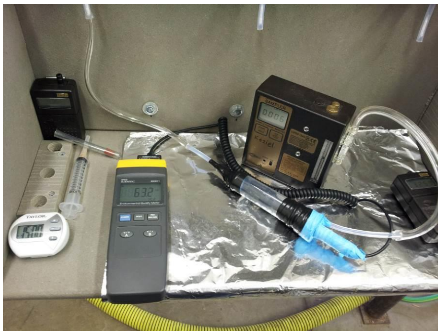
Figure 5. Pilot scale gas sampling station setup for relative humidity. Sample pump pulls air from the reactor vent line through sealed tube containing relative humidity probe.
