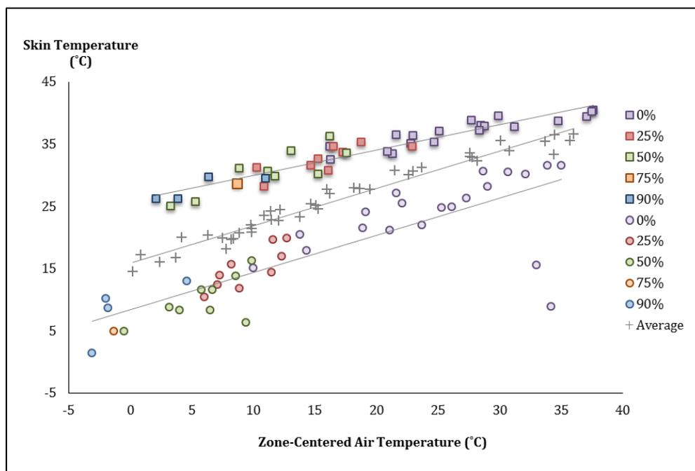
**Figure 21. Overall effects of trailer boarding variations (including 0-90%) on pig skin temperatures during transport. The maximum and minimum skin temperatures are plotted against zone-centered air temperature. The maximum skin temperature and the minimum skin temperature are represented by squares and circles, respectively. Different trailer boarding variations are represented by identical shapes with different colors. The average skin temperature is included on the figure as a reference.**
