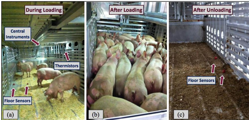
**Figure 14. Trailer interior conditions with instrumentation deployed and pigs present for (a) while loading, (b) after loading, before transport period, and (c) after unloading.**
