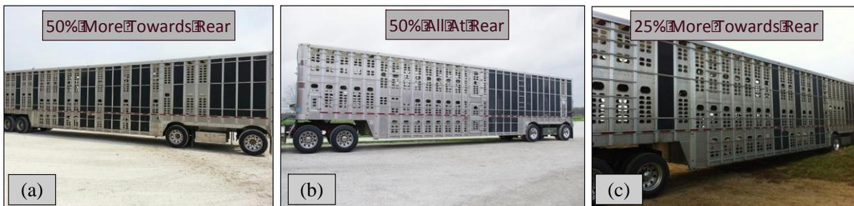
**Figure 12. Alternative boarding placement arrangements assessed for temperature -7 to 9°C (20 to 49°F). (a) 50% boarding more towards rear, (b) 50% boarding all at rear, and (c) 25% boarding more towards rear. Left indicates the front of the trailer and right indicates the back of the trailer.**
