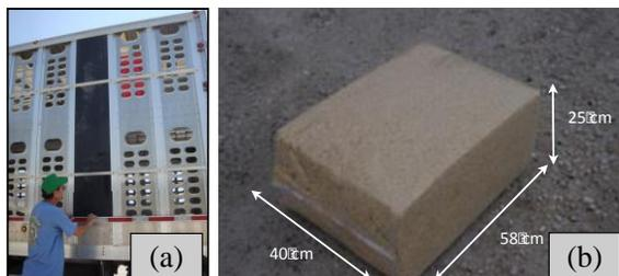
**Figure 10. Trailer management strategies for thermal environment inside the trailer during cool and cold conditions. (a) Boarding of the trailer by covering openings and (b) Substrate material (1 bag) that was scattered over the trailer floor prior to each monitoring trip.**
