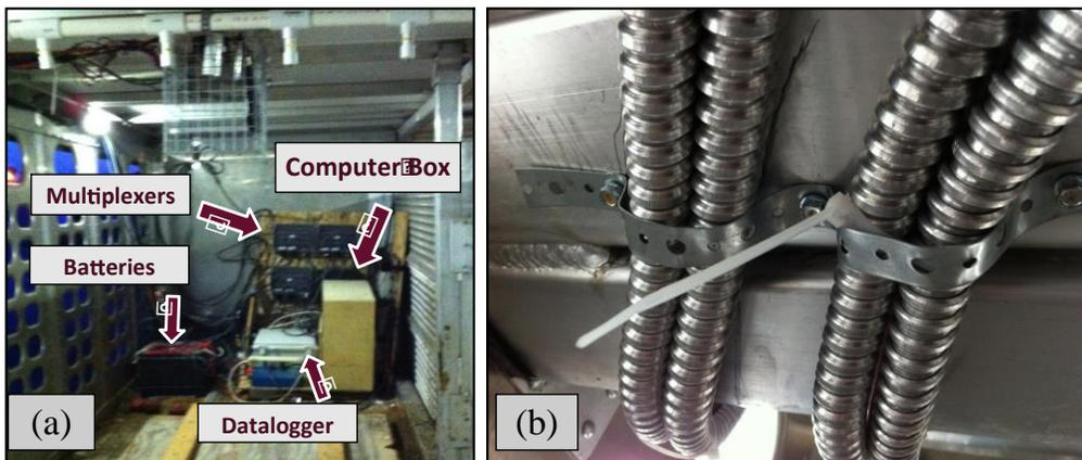
**Figure 5. Protection for instrumentation inside the trailer. (a) The protection of data acquisition center, of which consisted of a custom-fabricated computer box with a personal computer inside, three custom-fabricated multiplexers, one datalogger, and two parallel-connected batteries, and (b) the protection of flexible metal conduits for exposed instrumentation wires within the trailer.**
