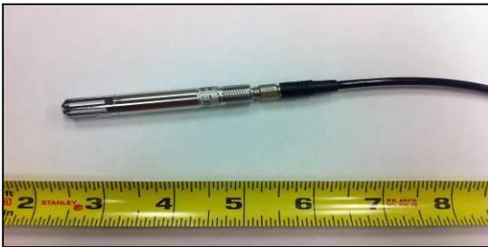
**Figure 7. Zone-centered air temperature and relative humidity (RH) sensor (Vaisala HMP60, Vaisala). Six zone-centered air temperature and RH sensors were implemented at the central area at the ceiling within each of the 6 cross-sections to measure the central air temperature and relative humidity of each trailer zone.**
