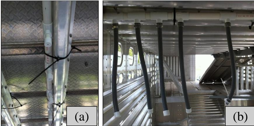
**Figure 3. Mounted PVC pipes for thermistors in trailer. (a) Mounted PVC on ceiling in front and rear zones, and (b) the PVC pipes fixed on the ceiling with 14 flex conduits hanging down. The vertical placement with respect to the height above the pigs' back was consistent for all zones within the trailer.**
