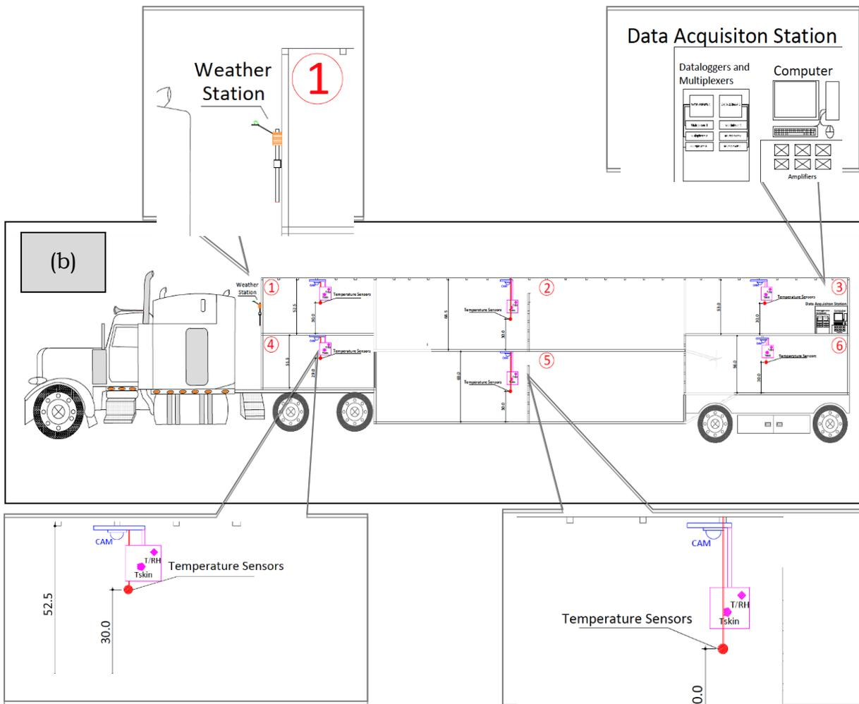
**Figure 2. Trailer Schematics. (a) Top zone and bottom zone illustrate the horizontal distribution of sensors in each zone and (b) the left-side elevation view of the six zones and illustrates the vertical distribution of sensors used to capture air temperature, skin temperature, zone-centered temperature/relative humidity and floor temperature.**
