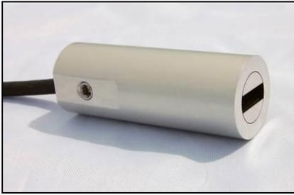
**Figure 8. Exposed surface temperature sensor (Apogee SI-111, Campbell Scientific, Logan). One infrared radiometer was implemented at the central ceiling within each of the 6 cross-sections to measure the exposed pigs skin surface temperature.**
