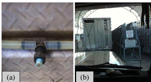
**Figure 13. Trailer management strategies for thermal environment of the trailer during warm and hot conditions. (a) Misting nozzles (TX-V626, Teejet Technologies) that were implemented inside the trailer, and (b) trailer location with respect to the fan bank when waiting to unload pigs at the plant.**
