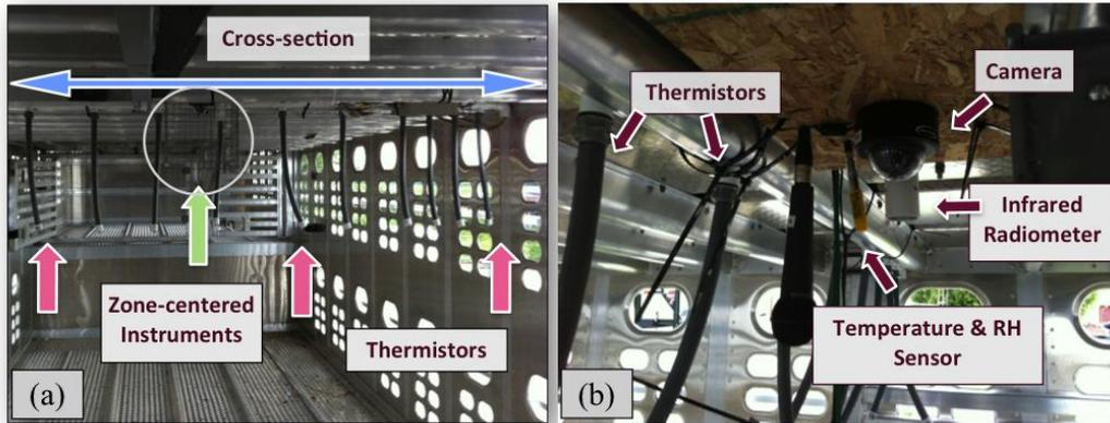
**Figure 4. Instrumentation location overview. (a) Trailer cross-section and (b) zone-centered instrumentation board. The zone-centered instrumentation board consisted of one connection box for thermistor sensors and one zone-centered air temperature and relative humidity probe, and one pig exposed surface temperature infrared radiometer.**
