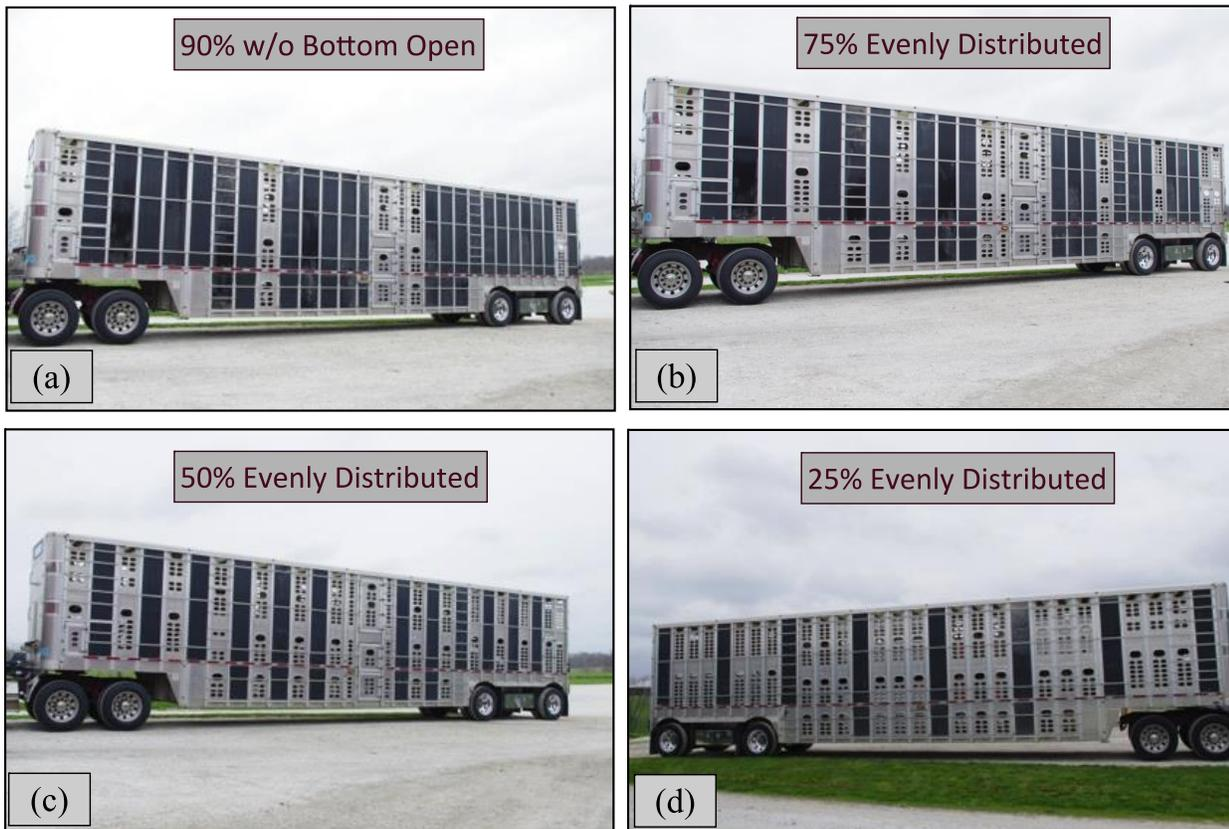
**Figure 11. TQA typical boarding percentage arrangements assessed for cold weather conditions. (a) 90% boarding with bottom covered, (b) 75% boarding coverage evenly distributed, (c) 50% boarding coverage evenly distributed, and (d) 25% boarding coverage evenly distributed.**
