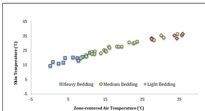
**Figure 20. Skin surface temperature versus corresponding zone-centered air temperature taken for different bedding depths, including measurements taken before transport, during transport and after transport during 43 monitoring trips over temperatures ranging from -14 to 38°C.**
