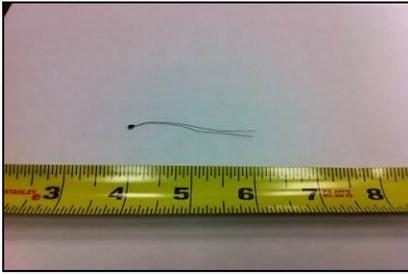
**Figure 6. Pig level air temperature sensor (Thermistor, Model No.10M5351, Honeywell Parts). Eighty-four thermistors were implemented in 6 cross-sections within each trailer zone to measure air temperature at pigs level, and located approximately 1.2 m above the trailer floor.**
