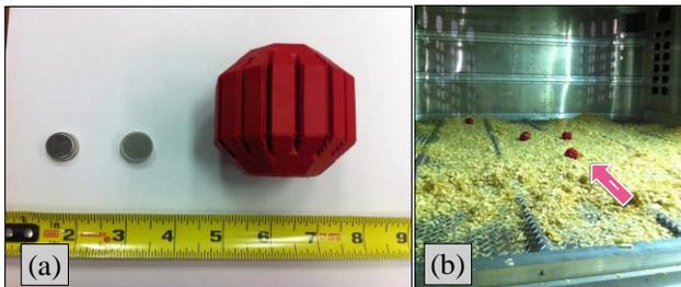
**Figure 9. (a) Floor/Bedding Temperature Sensors (iButton DS1921G-F5, Maxim, San Jose, CA) components, and (b) Three to six iButton sensors enclosed in protective rubber balls were placed on the bedding within each of the 6 zones at the start of transport to measure the floor/bedding temperature experienced by the pigs during transport.**
