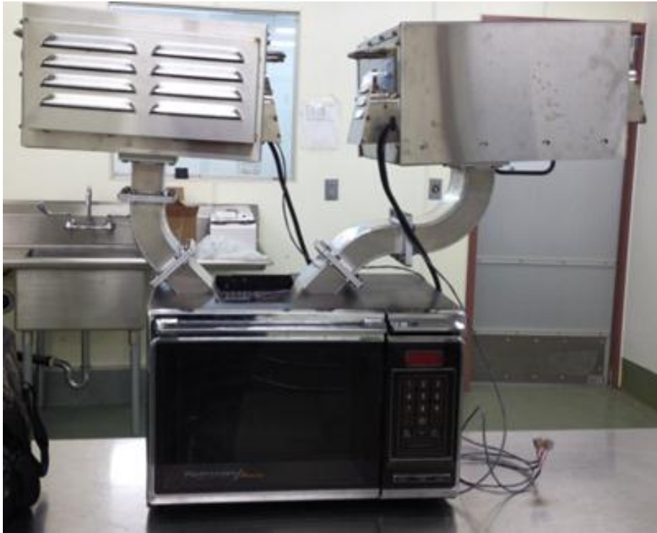
Figure 1. Dual generator electromagnetic unit utilizing two microwave power units, each containing one air-cooled 1.45 kW magnetron which develops 1,450 watts of continuous microwave energy at the 2,450 MHz frequency.
