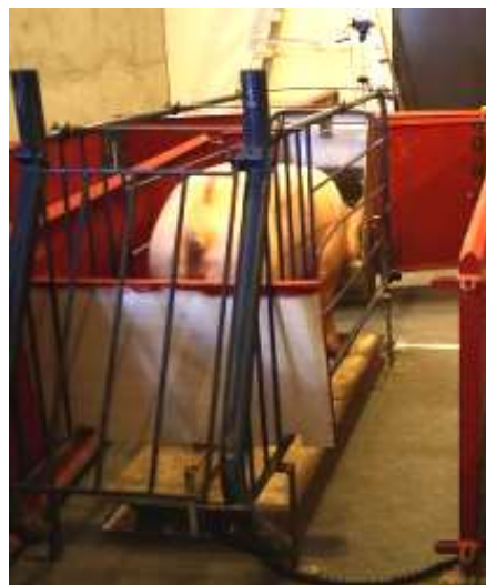
215 Figure 2. Data being collected on a sow embedded microcomputer-based force plate system
