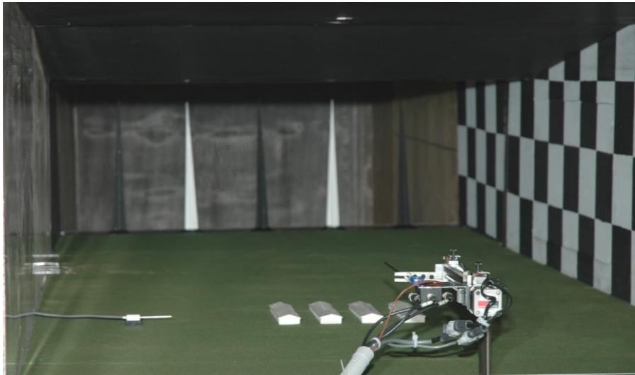
Fig. 7 Photo of 3D hot film anemometer behind four model swine finisher buildings mounted on vinyl mat. Spires are visible in background. Sensor to left of models is hot needle anemometer used to adjust air velocity at the height of the top of the building models.
