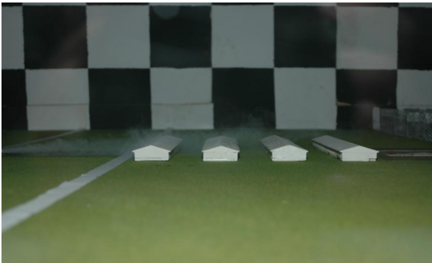
Fig. 14 Flow visualization showing smoke flow skimming across 4 swine finisher models perpendicular to air flow with a lagoon model 2h downstream. Air flow was 2 \text{ m s}^{-1} (5 mph).
