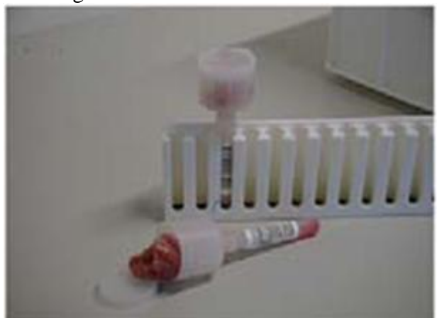
Figure 2. Example of specialized drip loss tube (manufactured and distributed by C. Christensen Laboratory, Denmark) and storage rack.
