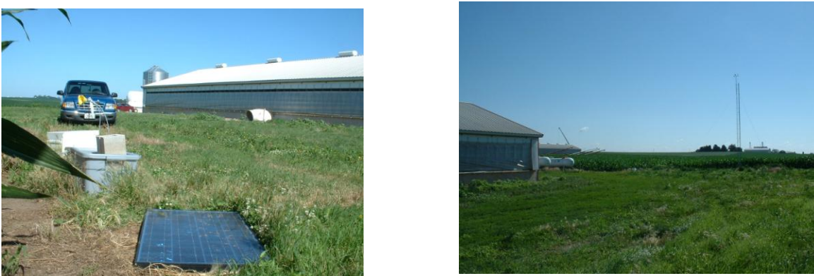
Figure 2. Complete collocated SPM set-up at one compass point and placement of the weather tower at a source.
