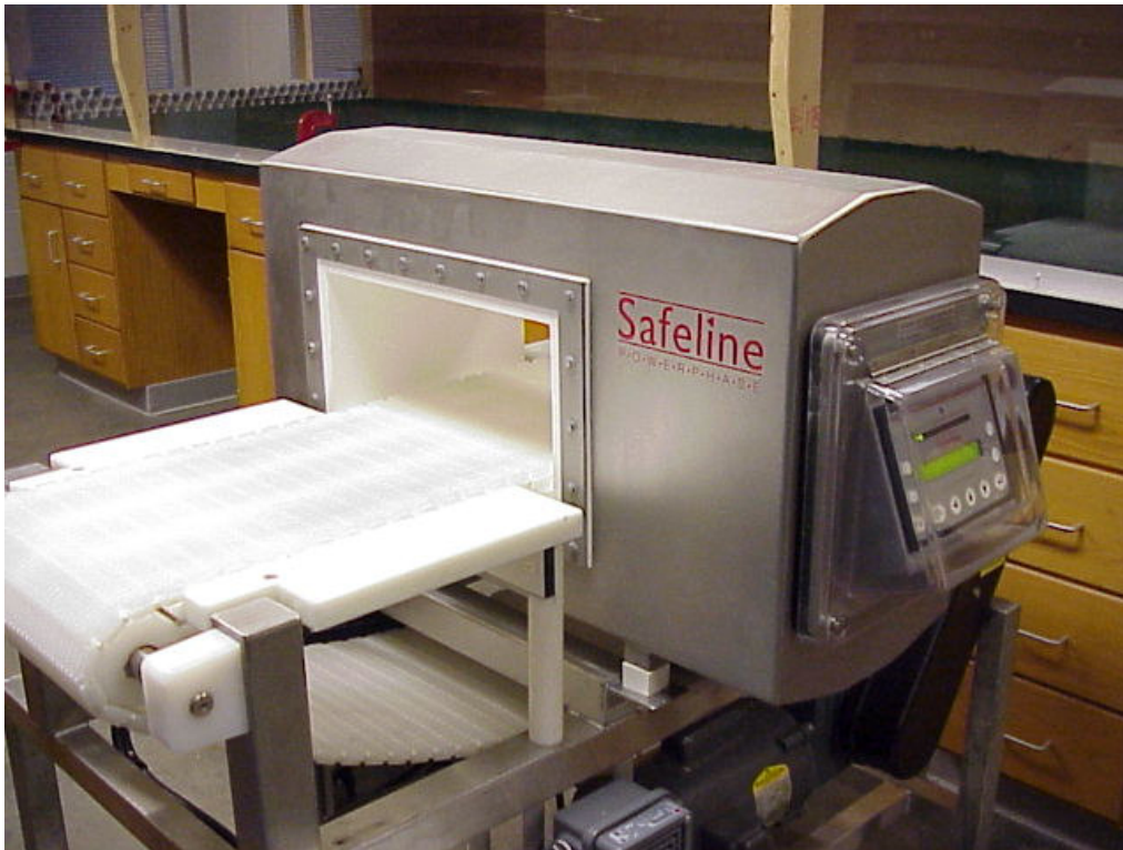
Figure 2. Safeline, Inc Power Phase metal detector used to conduct needle detection testing
