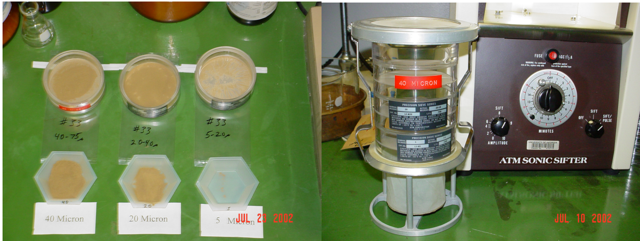
Figure 1. Sonic sifter apparatus used for separating the collected dust samples into small (5 to 20 \mu ), medium (20 to 40 \mu ) and large (40 to 75 \mu ) sizes.
